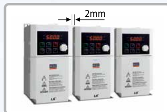
Side-by-side Installation (2mm between drives)
